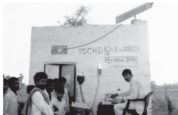
Fig. 5.12: Solar operated electronic milk testing equipment
