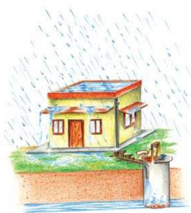
(b) Recharge through Abandoned Dugwell
