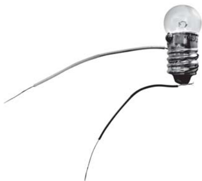
Fig.12.4 Bulb connected to two wires
